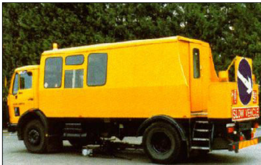
Figure 14 Deflectograph Survey Vehicle
